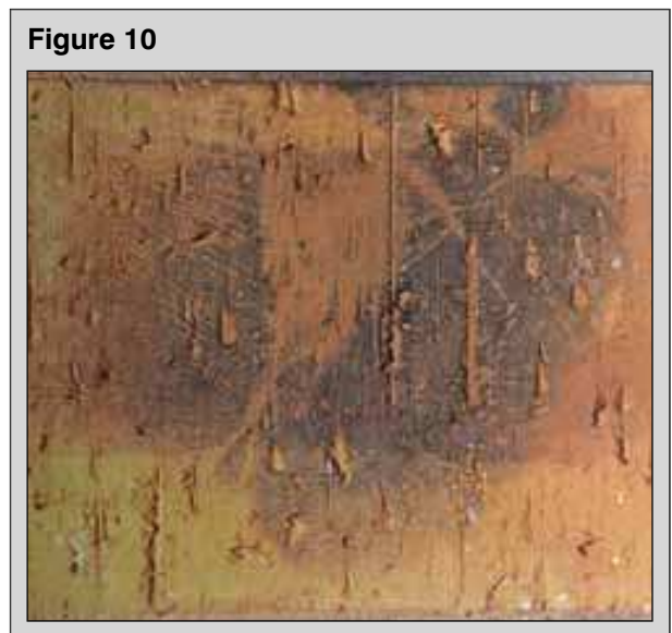
Figure 10. Ridge detail developed on a brick surface using an iodine-benzoflavone spray solution.
