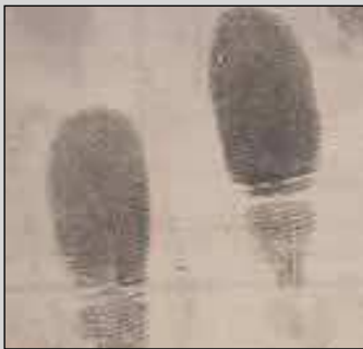
Figure 4. Latent fingerprints on paper after treatment with physical developer (PD). With this reagent, silver metal is deposited along the fingerprint ridges.
