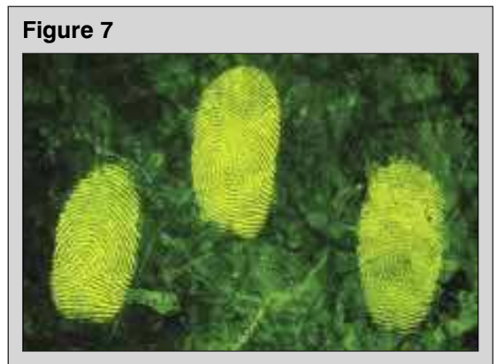
Figure 7. Latent fingerprints on white plastic after cyanoacrylate fuming and treatment with a luminescent stain (rhodamine 6G) – photographed in the luminescence mode under a high-intensity light source.
