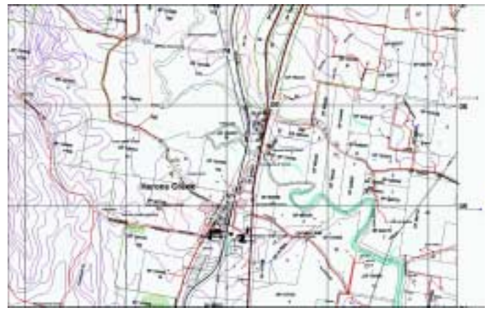
Figure 3b: Map side 2—This side of the map is lines, symbols and text only. No shading polygons are to be used except for large bodies of water. Contours are to be used. A full legend is included. (data sourced from field surveys and from project stakeholders.)
