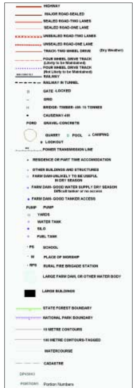
Figure 2: sample legend from a map generated from data coded to the Community Mapping standard. The standard covers the terms, symbols, symbol sizes and symbol colours.
